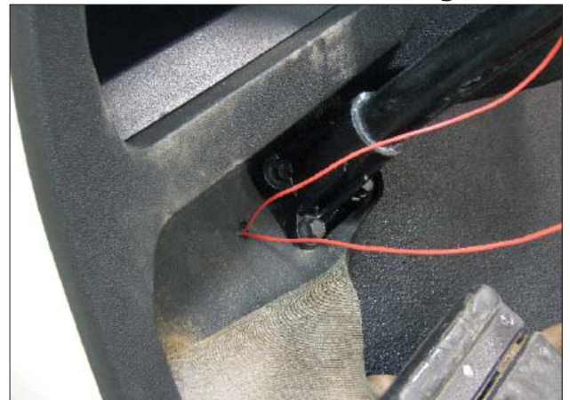
Wire Routing Through Floor for Steering Column Switch Mounting
